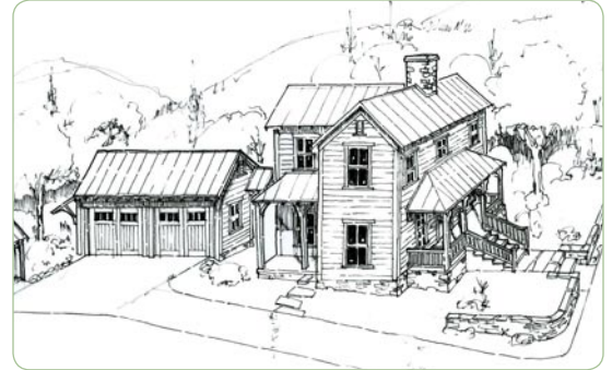
Images above: Large homes can best be created by the assembly of several one and two story volumes to create a disciplined plan arrangement that can be roofed over easily with style and restraint. In this way, the large ungainly roof masses of many contemporary tract and custom homes can be avoided where enormous roof volumes with multiple gables have to be fitted awkwardly over a sprawling plan arrangement of rooms.
