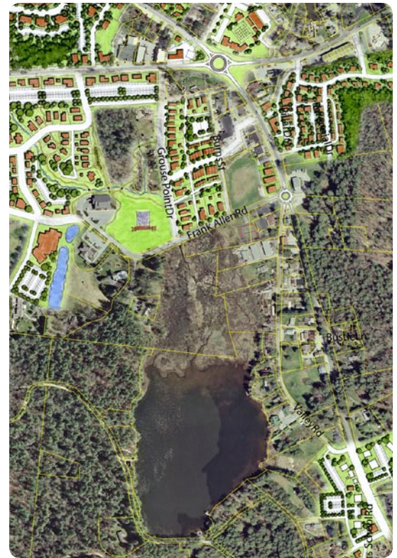
Cashiers Lake, shown in the plan above, serves as the retention pond for most of the crossroads. Through the years, the lack of a stormwater management plan has caused the lake to become heavily silted.
