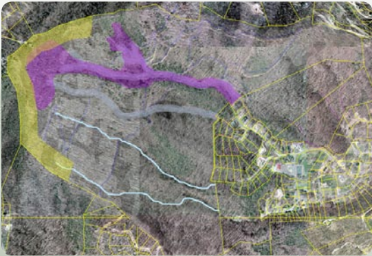
An existing conditions diagram that illustrates streams, buffers, and floodplains to be avoided.
