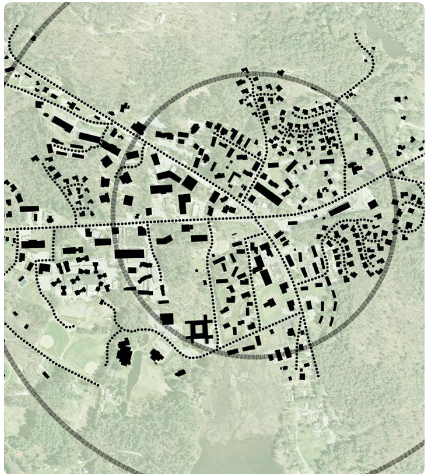
Existing buildings and road network illustrating the relatively small size of most of the buildings and the limited street connections
