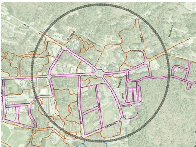
Proposed pedestrian network for Cashiers including paved walkways (magenta) and trails (orange). The circle represents 1/4 mile radius (5 minute walk) from the main intersection.
