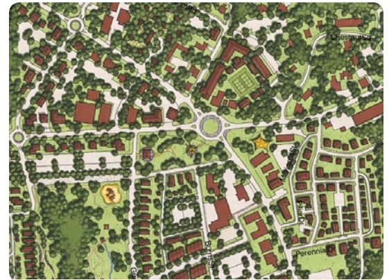
Roundabouts and new street connections provide context-sensitive solutions for increasing safety and walkability and decreasing traffic volumes in the Cashiers crossroads area.
