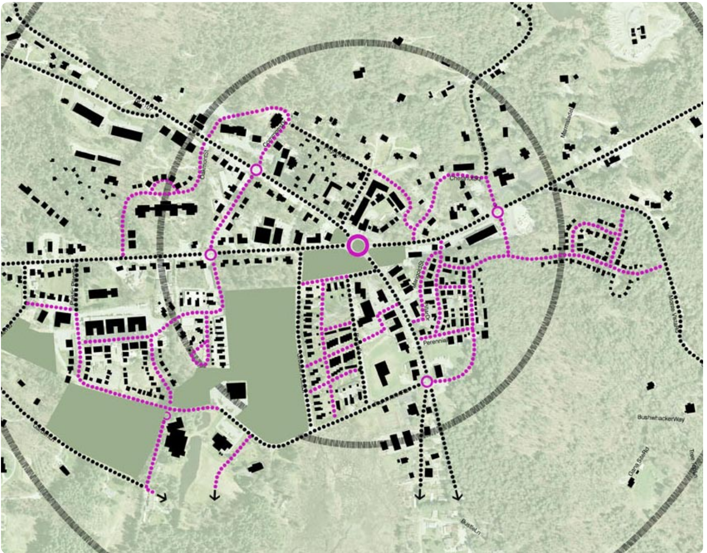
Figure Ground Diagram illustrating the 2027 Concept Plan of infill development, new road connections, and public open spaces
