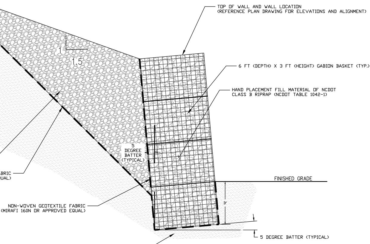
placement will require supplementing with handwork to ensure the desired results. The cells in any row shall be filled in stages so that the depth of rock placed in any one cell does not exceed the depth of rock in any adjoining cell by more than 12 inches. Along the exposed basket faces, the outer layer of stone shall be carefully placed and arranged by hand to ensure a neat, compact placement with a uniform appearance.
