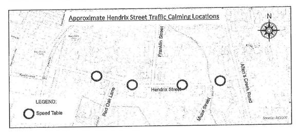
NOTE: Drivers might try to avoid speed tables by swerving onto the grass shoulder. Luckily, Hendrix Street has some curb and gutter sidewalks and street trees that will limit this behavior. If speed tables are installed where there is a grass shoulder, it is recommended that an advisory sign, a flexible bollard, or other vertical element be placed in the shoulder to further limit this potential behavior.
