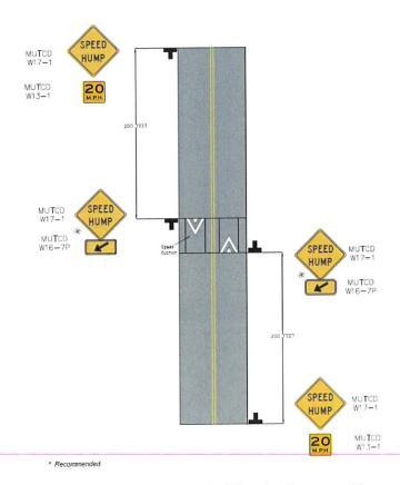
NOTE: Speed limit advisory signs are only recommended for the first speed hump in the series from each direction on Auburn Street. However, MUTCD signs W17-1 and W16-7P are recommended for all speed humps, as they provide visibility at each location.
