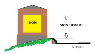
The height of a sign is measured from the highest point of a Sign Face to the highest adjacent grade at the base of the sign. The height of the sign structure shall not exceed the height of the Face by greater than twenty percent (20%).
